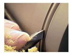
starting at the side and turning to the top. This tool can be used on a piece that would be hard to reach with a spindle gouge.
